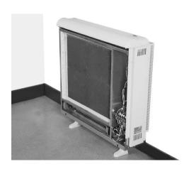
13.- Refit the inner front panel. If the bricks have been fitted correctly you will have no difficulty in refitting the panel. Make sure the bottom edge of the inner panel is inside the front lip of the heater. Please see below
