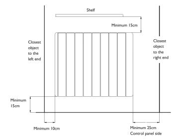
Position and fix the brackets at the correct distance from the floor. It is possible to use the radiator as measuring unit by positioning it on two polystyrene package elements and placing two supports above as indicated on the figure:
