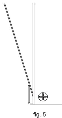
12. Attach the front panel by hanging it on the "V" in the upper part and securing it at the bottom with the two screws.
